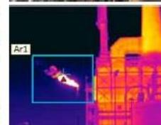
Although invisible to the naked eye a thermal imaging camera can monitor whether a flare is burning or not. If the flare is not burning, harmful gasses can enter the atmosphere, an alarm can go off and immediate action can be taken.
