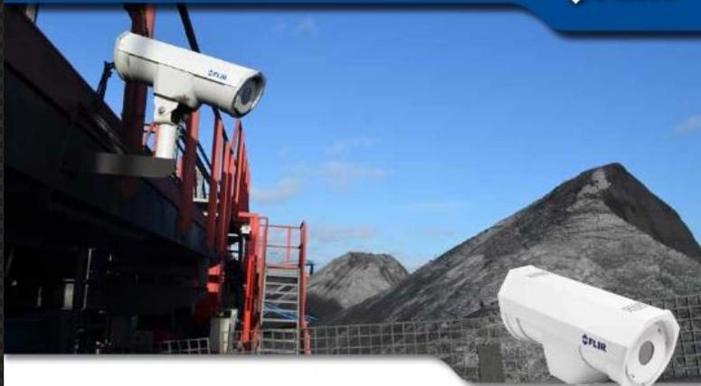
FLIR cameras enable timely detection and localization of self-combusting coals.
