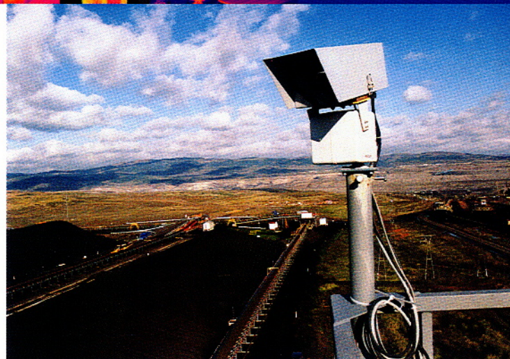
The FLIR Systems ThermoVision™ infrared camera mounted on a mast over the coal piles of the Nástup Mines Cooperation in the Czech Republic.
