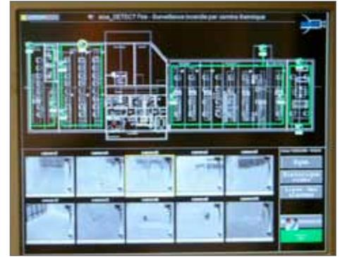
The touch screen interface shows the floor plan of the facility and live thermal video footage of all ten FLIR A310 thermal imaging cameras, including automatic alarms and accurate temperature readings.
