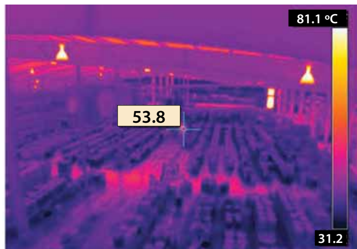
A subsequent image of the same area shows that the abnormal reading has increased further, causing an alarm to go off.
