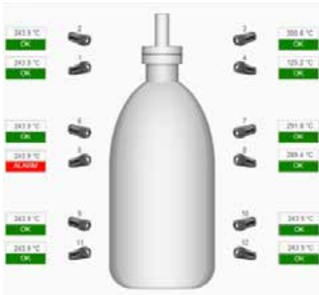
24 thermal imaging cameras from FLIR are located near the gasifiers, in order to look at the spots of the most interest for the analysis.
