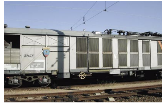
The "Vulcain" SNCF test wagon, which in future will carry the infrared camera to inspect catenaries.
