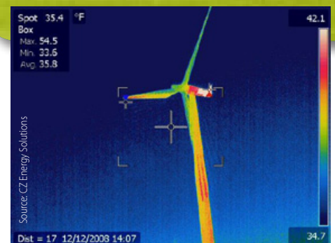
A thermal image of a wind turbine taken from ground level
