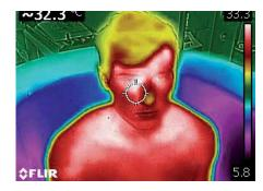
The FLIR AX8 continuously monitors the patient's upper body temperature and displays it on a patient screen, installed on top of the cabin, as well as on a display monitor outside of the cabin.
