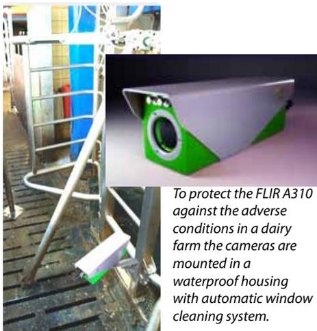
To protect the FLIR A310 against the adverse conditions in a dairy farm the cameras are mounted in a waterproof housing with automatic window cleaning system.
