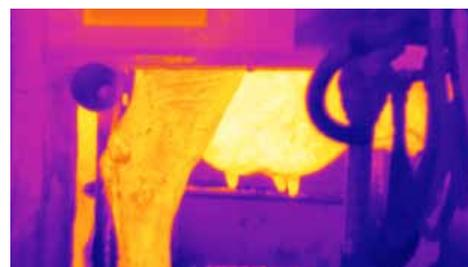
The two FLIR A310 thermal imaging cameras record images of the cow's udder from both sides.
