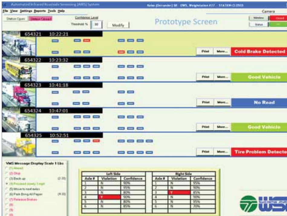
AIRS detects inoperable brakes (left) on this commercial vehicle.
