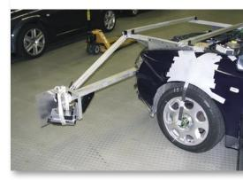
Infrared camera ready to measure rolling resistance and other tyre features
