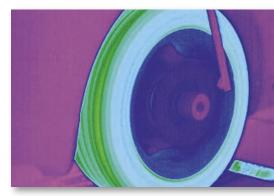
On the tyre testbed: infrared camera detects rolling resistance and heat development of tyre
